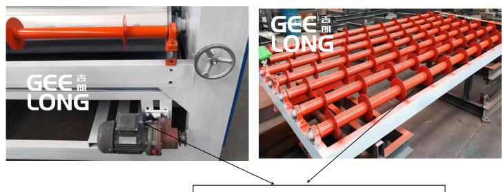
Reducer machine plus disk conveyor for glued veneers unloading, more good support for unloading
